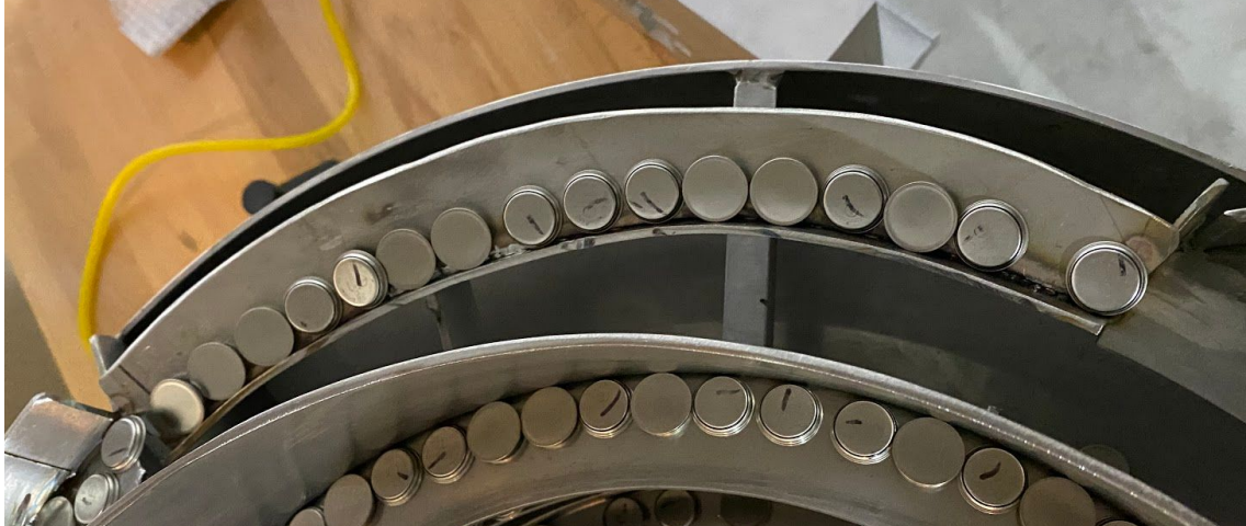
Modified Rail for iButtons to feed to the Orientation Check.
